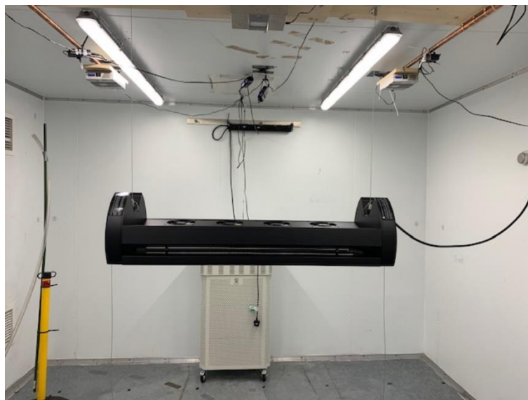
Plate 2 Sanilume Air device suspended from the ceiling in the chamber at mid-height
